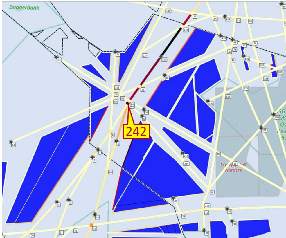
Figure 29: Waypoint collision risk of scenario A1 for the modelled area (percentage basis)
