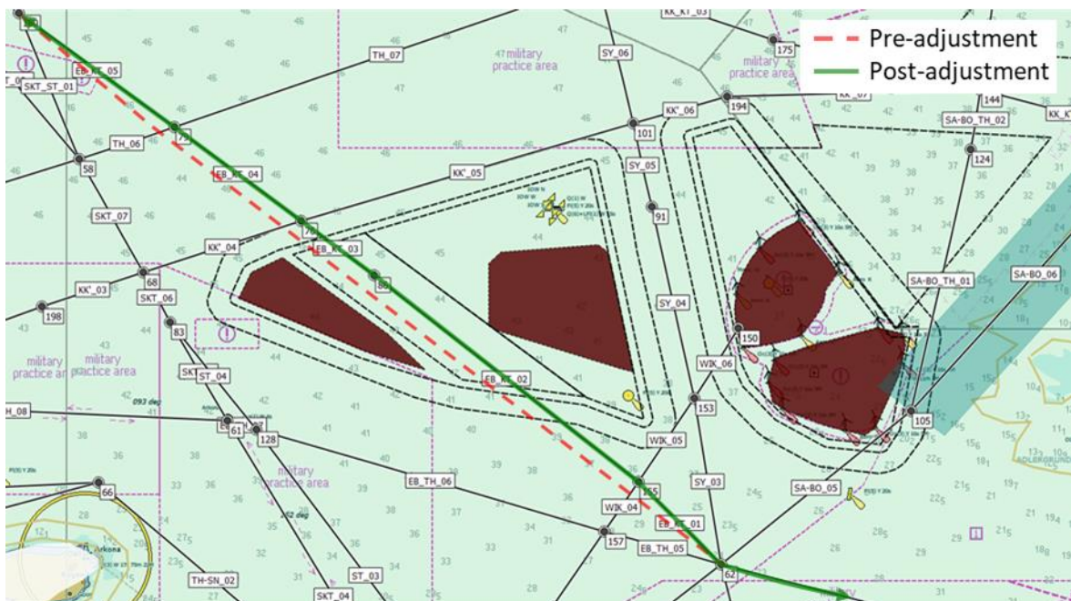
Figure 30: Adjustment to the centreline of the traffic navigating from The Sound to Adlergrund TSS
