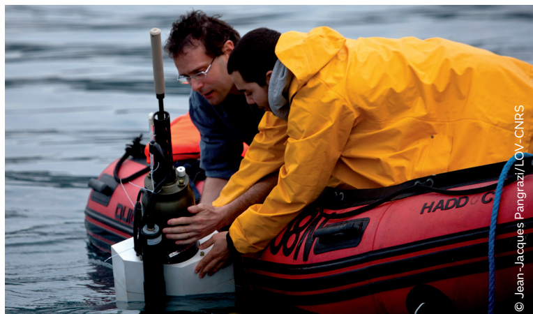
Deployment of a BGC float, equipped with 6 biogeochemical sensors.
