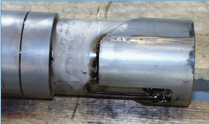
Fig. 2: Damaged plunger of injection pump
