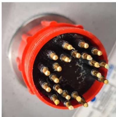
Picture # 5 - SubConn connector in a very good condition (SN 224)
