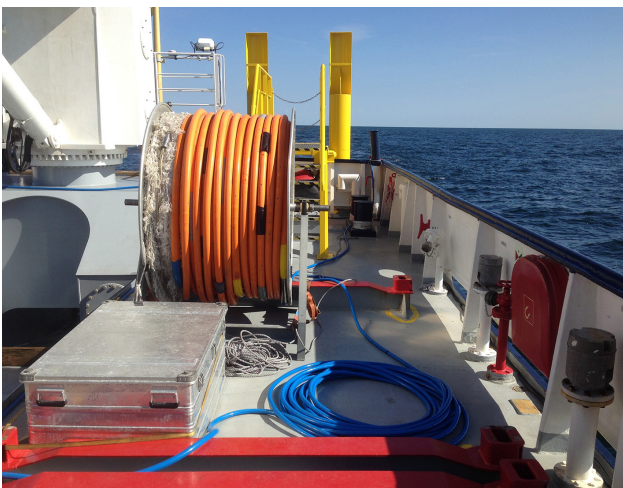
Looking aft across working deck of offshore support vessel LEV TORNADO at the multichannel seismic streamer winch. (Photo: Florian Meier, Fraunhofer IWES)
