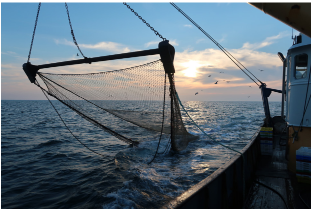
Standard gear for surveying fish according to StUK4: 7 m beam trawl on the starboard outrigger of a shrimp cutter chartered for the site investigation of the protected asset fish. (Photo: Sebastian Fuhrmann, BSH)
