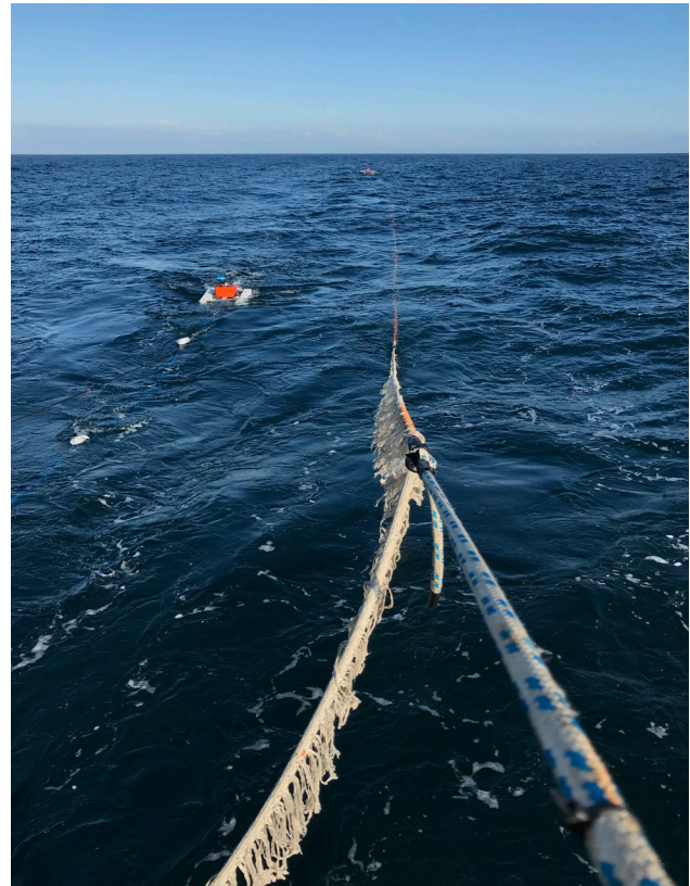
On the right, the multichannel seismic streamer; on the left, the sparker source with the GPS case. (Photo: G. Frielinghaus, Fraunhofer IWES)
