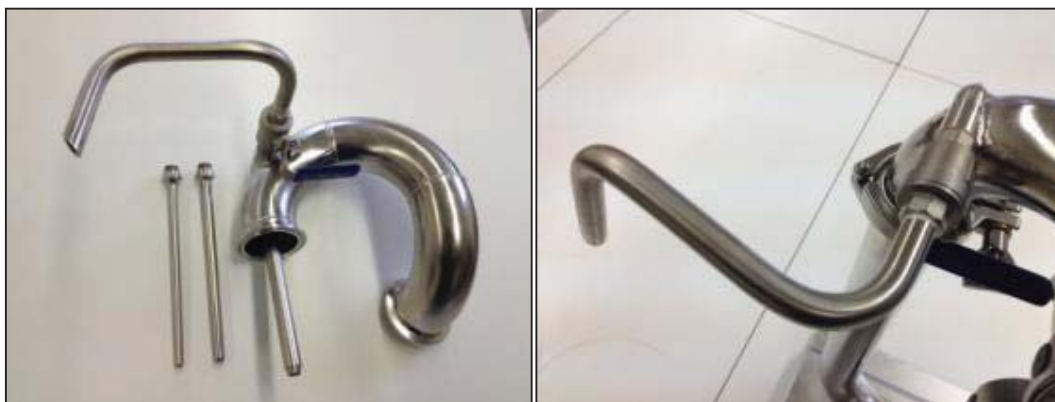
Figure 2: The isokinetic bypass sampling port, dismantled (left) and installed (right)
