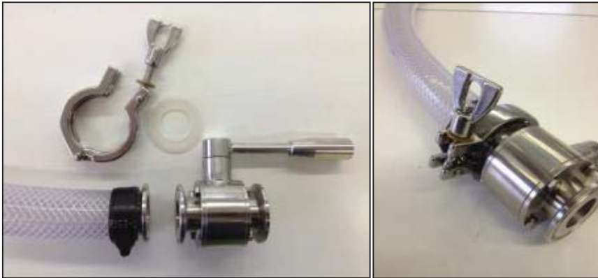
Figure 3: The connecting system and additional ball valves
