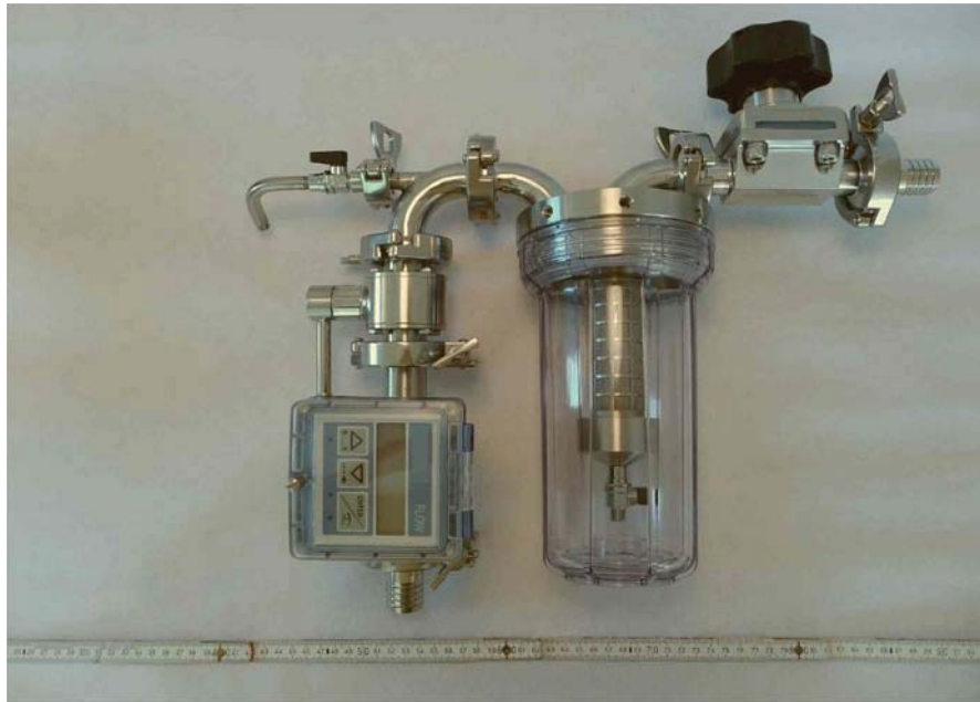
Figure D.1: Triton NP 6007 TG 18 skid: basic set of elements
