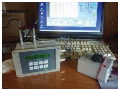
Figure 1: PAM fluorometry; a fast method to determine (bulk) phytoplankton biomass and the photosynthetic activity of the phytoplankton. Left Universal Control Unit, right Water ED/B
