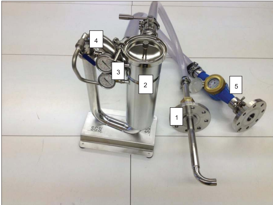
Figure 1: The SGS Ballast Water Sampler v02. The parts are numbered in the order that the water passes through the sampler. 1: Sampling pipe. 2: Filter housing. 3: Pressure gauges. 4: Bypass sampling port. 5: Volume count.
