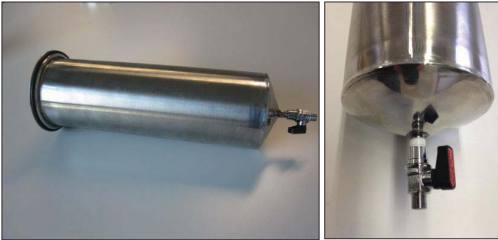
Figure 7: The stainless steel screen filter inlet of the SGS BWS1, the rubber ring at the top prevents water and organisms from bypassing the filter. The valve at the bottom allows easy collection of the sample.
